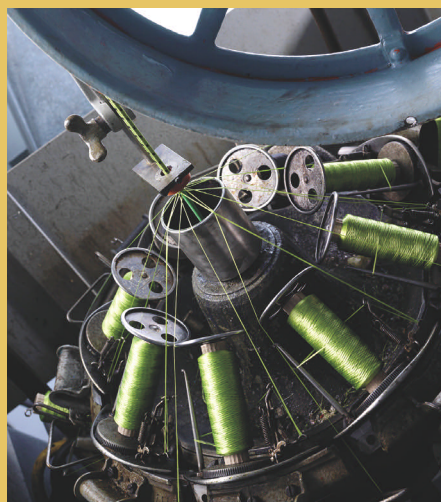
A spinning machine makes cable from spools of wire and thread.
