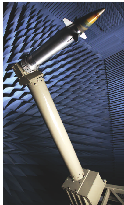
FIGURE 3. A mechanical arm rotates an antenna under test around a pivot point. Courtesy of Tyco Electronics.
