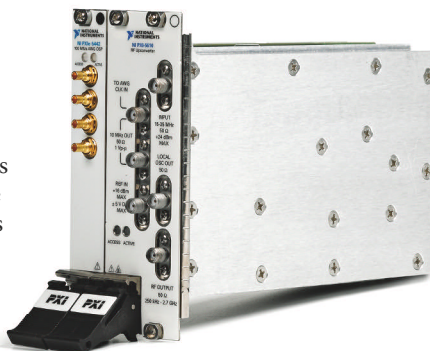
The PXI Express bus allows instruments such as this vector signal generator to stream data off a disk array and provide hours of test stimulation. Courtesy of National Instruments.
